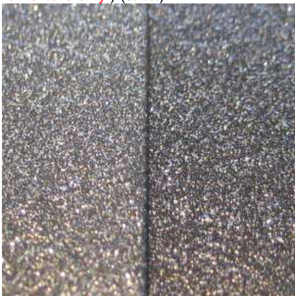
Picture 5: Makro impression of two MetallicEffect surfaces (illumination optimized for texture only!) (Schüco)
